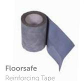
Reinforcing Tape is 150mm wide self-adhesive waterproofing tape for sealing critical details such as wall junctions, soap recesses, pipe boxing and other such areas prior to tiling. Choose either Tilesafe or Floorsafe versions according to the Floor Membrane Kit selected.
