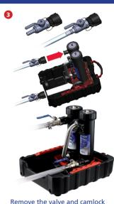
assembly from the parts box and attach to existing hose either rom the MagnaCleanse connection kit or hose from your existing PowerFlush machine.
