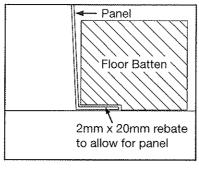
4. Fit the front panel by inserting the lip under the rim of the bath. Secure to the wall and floor battens with suitable screw fixings (not supplied).
