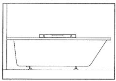
2. Measure the dimensions A and B as illustrated on the bath and mark onto the *front panel*. Note: the *kick strip* is to be used for any adjustment to the height of the *front panel*, not the lip. Also make sure the *front panel* is the correct way up and facing the correct direction before marking.
