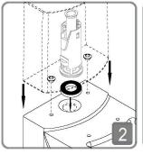
Place doughnut washer onto syphon and lower cistern into place.
