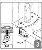
Tighten cistern onto WC as per diagram B-B.
