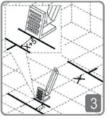
Position fixing bracket in the required position on the floor.
