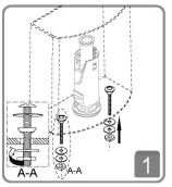
Fix fitting bolts into cistern as per diagram A-A.
