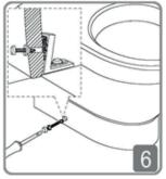
Fix WC to fixing bracket using screws supplied.
