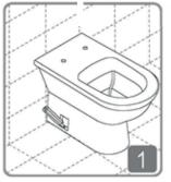
Place WC into position required and mark floor through fixing holes. This mark will show the drilling points.
