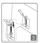
Place WC back into position, ensuring plumbing connection are water tight and fix WC to floor.
