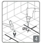
Drill into the floor using a 9mm drill bit. Insert wall plug into the hole.
