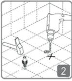
Drill into the floor using a 9mm drill bit. Insert wall plug into the hole.
