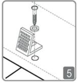
Install fixing bracket to floor with fixings supplied.
