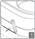
Place WC into position and mark the floor around the edge of the WC. Mark floor level with the fixing hole.
