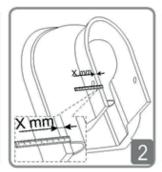
Remove WC and measure thickness of ceramic where the fixing hole is positioned (X).
