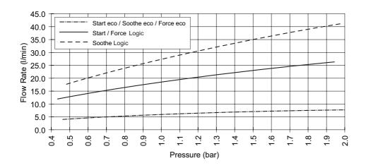
To cap the flow rate at a maximum of 7 litres per minute, or to reduce any vibration caused by certain water systems, an optional flow regulator is provided. If required, install the flow regulator between the shower outlet and the hose, as illustrated.
