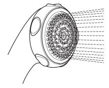
Soothe: Turn the spray plate anticlockwise until it 'clicks'. Water will flow from the large diameter holes.
