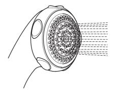
3. Force: Turn the spray plate anticlockwise until it 'clicks'. Water will flow from the inner set of holes.
