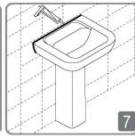
Using an appropriate sealant, seal washbasin to the wall.
