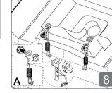
Before commencing with the fitting of the half pedestal make water connections. Then insert half pedestal spring fixing as shown in diagram A.
