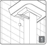
Position washbasin into desired position and ensure washbasin is level. Mark fixing points onto the wall.
