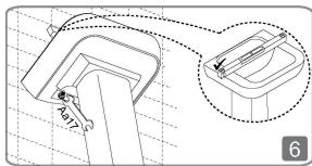
Ensure the washbasin is level and tighten nuts to ensure washbasin is secured to the wall.
