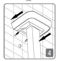
Position basin onto fixing bolts and make water connections.
