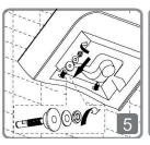
Insert washers and fixing nuts onto bolts as shown in diagram.
