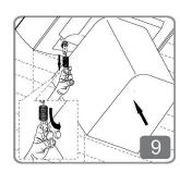
Insert hook into hole in half pedestal.
