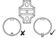
Place the accessory over the wall plate with the locking grub screw at the bottom. Tighten locking grub screw using the correct sized screwdriver.
