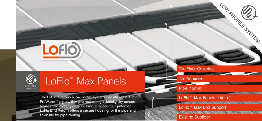
LoFlo™ Max is a low profile solid floor system that will increase floor height by as little as 18mm. The dry screed board acts as a heat conducting surface transferring heat from the pipe to the floor covering achieving excellent heat
