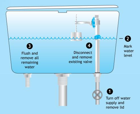
Valve can be fitted on either side of cistern.
